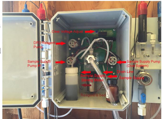
3. Make sure DPD pump is primed by turning it on in the TrueDPD Manual menu on the controller. You will see it getting pumped into the sample cell. About 5 seconds and turn off. Next, make sure sample supply lines are connected and control valves at flow cell are open then flush out sample by turning on flow in same menu for about 10 seconds. (you will see a small stream of fluid coming out the drain tube)
