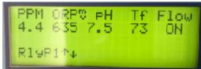
These readings show a free chlorine reading well above minimum standards but with 100 ppm of cyanuric acid. This pool has a problem with yellow algae that would most likely not exist with proper ORP levels.
