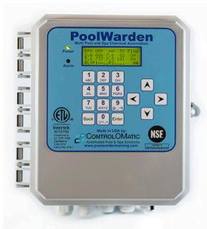
1 or 2 pool Free Chlorine/ORP/pH controller with temperature monitoring and EnergySmart heater control with AUX relays (2 per pool) which also allows for controlling salt systems or ancillary chemicals. Data recording and security. Langelier Index, NSF 50, UL
