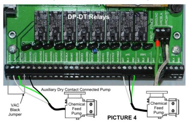
No voltage is being supplied to the load / equipment when the relay is off, hence, voltage is being supplied to the load / equipment when the relay is on. Any standard chemical feed pump or solenoid can be hard wired directly into the appropriate ORP and pH connection terminals as shown below in PICTURE 4 so long as their voltage matches the input VAC connected to the PoolWarden.
